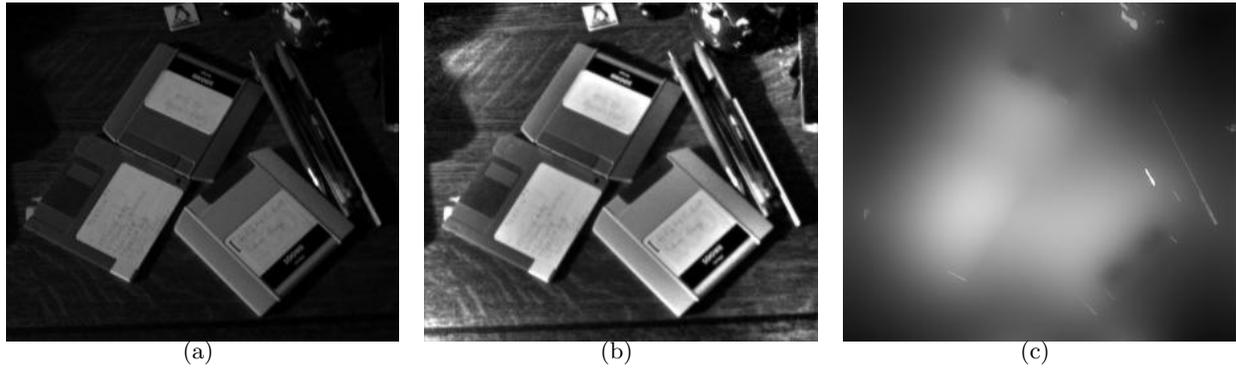
Figure 2. The result of gray image by proposed method. (a) the observed image. (b) the reflectance image. (c) the illumination image.
