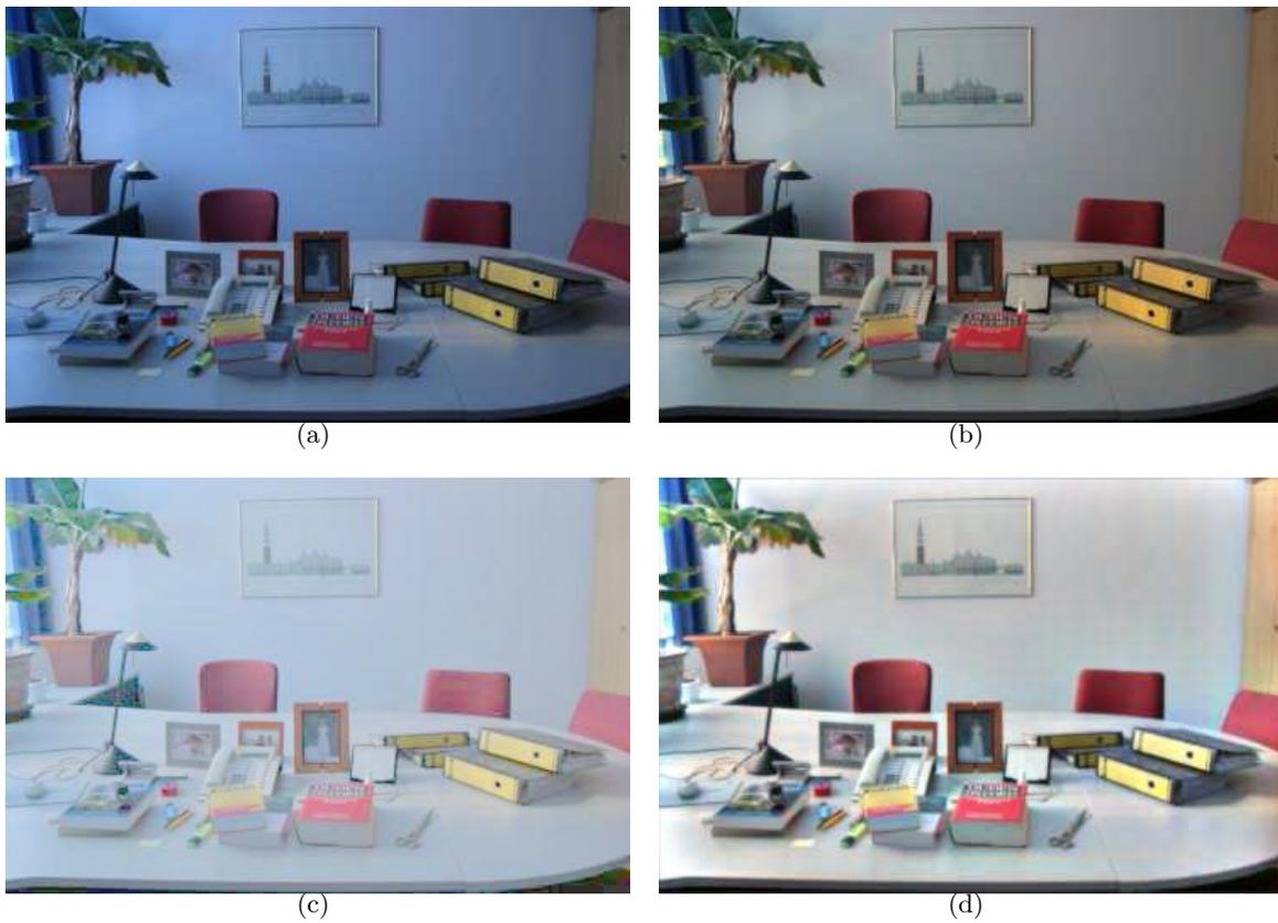
Figure 3. The comparison of different methods. (a) the observed image. (b) the grey-world assumption. (c) MSRCR.<sup>6</sup> (d) the reflectance image by proposed method.
