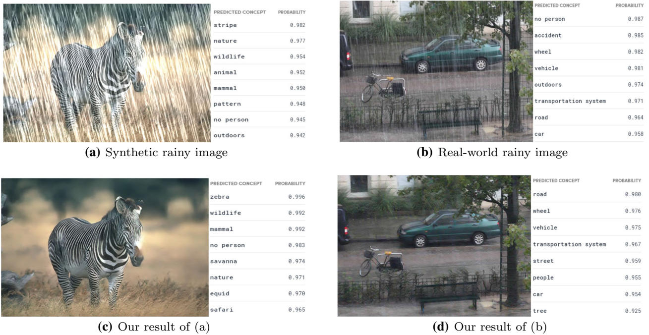
Fig. 21 Preprocessing for image recognition on the Clarifai platform. a and b are recognized as “stripe” and “no person” with the highest probability, respectively. c and d , i.e., our results are accurately recognized as “zebra” and “road” with the highest probability, respectively
