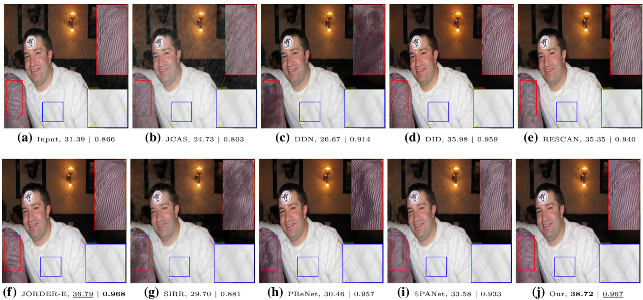
Fig. 9 One visual comparison with PSNR | SSIM values from the synthetic data set ‘ DID-Data ’
