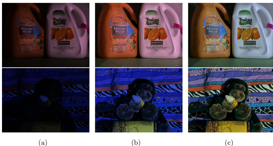
Fig. 17. Color distorted images. (a) Input images; (b) directly enhanced results; (c) results of adding gray-world algorithm with the proposed algorithm. (For interpretation of the references to color in this figure caption, the reader is referred to the web version of this paper.)
