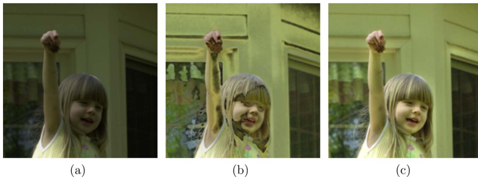
Fig. 5. Example of fusion strategies. (a) Input image; (b) enhanced result by naive fusion; (c) enhanced result by multi-scale fusion.
