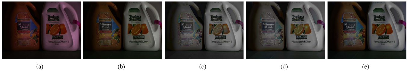
Fig. 7. Comparison of color correction. (a) The observed image; (b) the ground truth; (c) the result by Kimmel's method [29]; (d) the enhanced image by Ng's method [30]; (e) the result by the proposed method.
