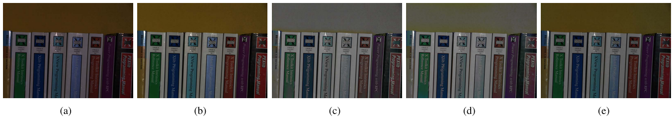
Fig. 8. Comparison of color correction. (a) The observed image; (b) the ground truth; (c) the result by Kimmel's method [29]; (d) the enhanced image by Ng's method [30]; (e) the result by the proposed method.
