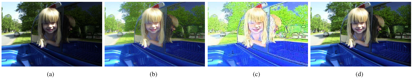
Fig. 11. Comparison of reflectance estimation. (a) The observed image; (b) Gamma correction with the reflectance directly derived from Ng’s method [30]; (c) Gamma correction with the reflectance directly derived from Bayesian method [37]; (d) Gamma correction with the reflectance directly derived from the proposed method.
